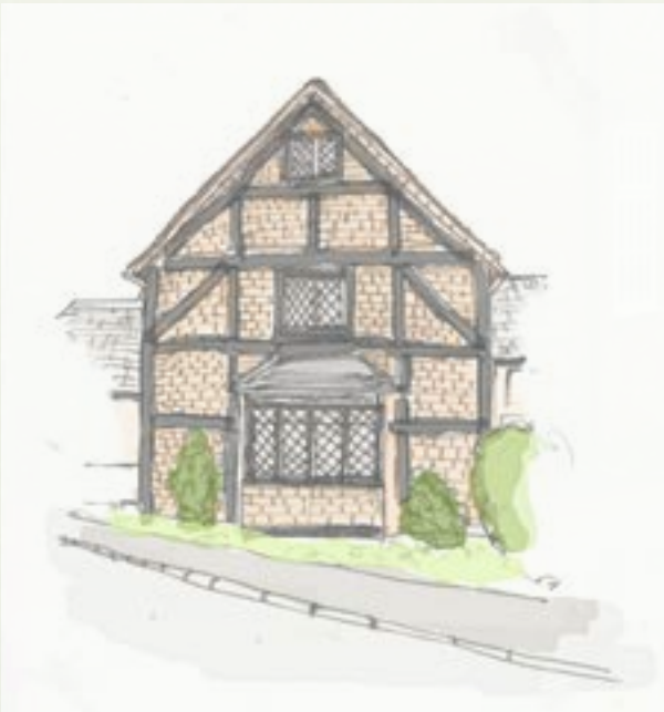
(Figure 9: Timber Frame Brick Infill Gable)
